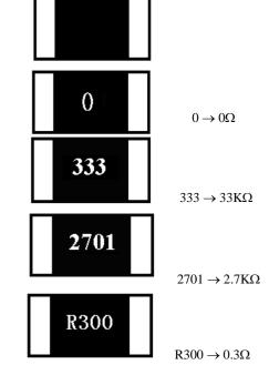
4.6 Standard E-96 series values of HP03≤±1%: due to the small size of the resistor's body, 3 digits marking will be used to indicate the accurate resistance value by using the following multiplier & resistance code.
